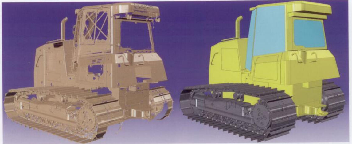
3D scan and final 3D model of the tractor
