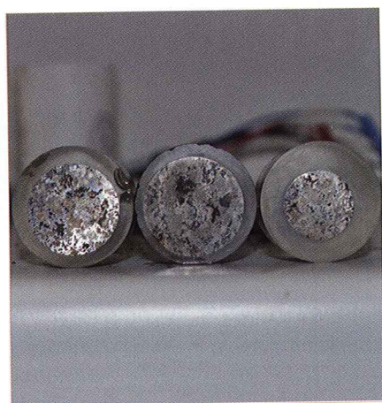
Mild steel and cast iron samples following exposure to the electrochemical test cell for corrosion rate measurements.
