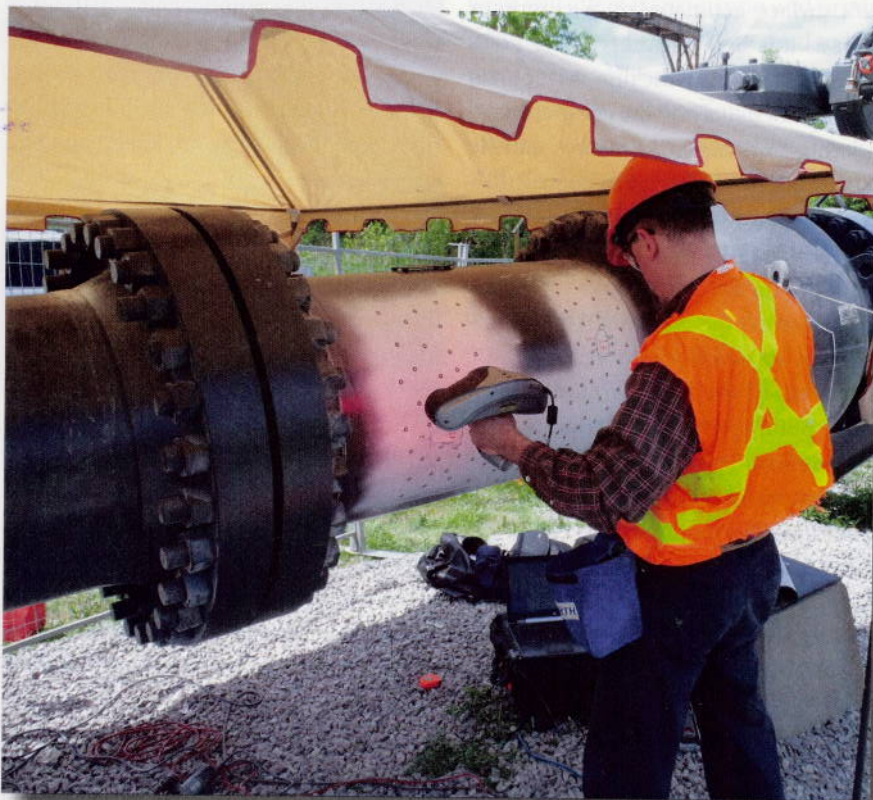
An inspector at a refinery uses the handheld 3-D scanner on a pipe segment to conduct a direct assessment of external corrosion. Photo courtesy of Creaform.
