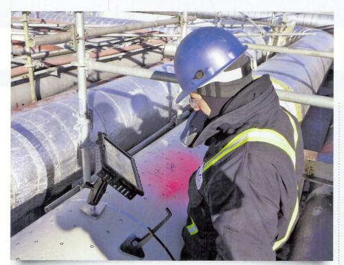
ultrasonic and pit gauge testing. The latter also measures the depth of corrosion or damage—often, dents—in a pipeline or pressure vessel.
